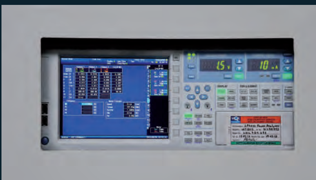
Efficiency determination as per IEC 60034-2-1 : 2024
